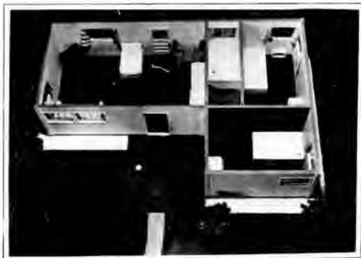
A typical Fort Wayne House. The shell of the house can be erected in two hours. It can be dismantled and moved to another site. The interior arrangements are shown in the plan and the model below. It will be noted that there is a large living room with one end equipped with kitchen equipment and heating stove. The two bedrooms are small, and are provided with open-front closets which may be entirely closed with curtains.
